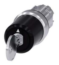
Key-operated switch BKS, 22 mm, round, metal, shiny, lock number S1, with 2 keys, 3 switch positions I-O<II, left latching, right momentary contact type, actuating angle 2x45°, 10:30h/12h/13:30h, key removal O+I, with laser labeling, upper case and lower case, always upper case at the beginning of the word
