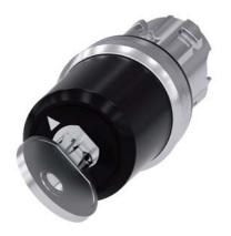
Key-operated switch BKS, 22 mm, round, metal, shiny, lock number S1, with 2 keys, 2 switch positions O<I, momentary contact type, Actuating angle 45°, 10:30h/12h, key removal O, with laser labeling, upper case and lower case, always upper case at the beginning of the word
