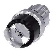
RONIS key-operated switch, 22 mm, round, metal, shiny, lock number 455, with 2 keys, 2 switch positions O-I, latching, actuating angle  $90^\circ$ , 10:30h/13:30h, key removal O+I, Z=50-unit packaging
