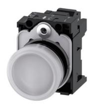
Indicator lights, 22 mm, round, plastic, white, lens, smooth, with holder, LED module, with integrated LED 110 V AC, spring-type terminal, with laser labeling, upper case and lower case, always upper case at the beginning of the word
