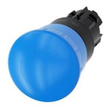
Mushroom pushbutton, 22 mm, round, plastic, blue, 40 mm, positive latching, acc. to EN ISO 13850, rotate-to-unlatch, with laser labeling, upper case and lower case, always upper case at beginning of line
