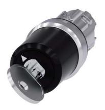
key-operated switch Siemens, 22 mm, round, metal, shiny, lock no. STGH10, with 2 keys, 2 switch positions O-I, latching, actuating angle 90°, 10:30h/13:30h, key removal O+I, with laser labeling, upper case and lower case, always upper case at beginning of line
