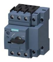
Circuit breaker size S00 for motor protection, CLASS 10 with overload relay function A-release 2.2...3.2 A N release 42 A screw terminal Standard switching capacity
