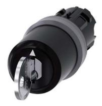
Key-operated switch IKON, 22 mm, round, plastic with metal front ring, special lock, with 2 keys, 3 switch positions I>O<II, momentary contact type, actuating angle 2x45°, 10:30h/12h/13:30h, Key removal O
