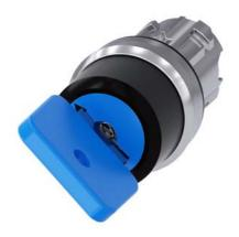
Key-operated switch O.M.R, 22 mm, round, metal, shiny, lock number 73038, blue, with 2 keys, 2 switch positions O-I, latching, actuating angle 90°, 10:30h/13:30h, key removal I, with laser labeling, inscription or symbol Customer-specific selection with SIRIUS ACT configurator (CIN)
