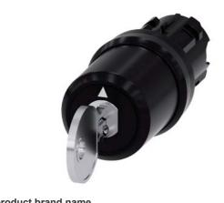
key-operated switch Siemens, 22 mm, round, plastic, lock number SSG10, with 2 keys, 3 switch positions I-O-II, latching, actuating angle 2x45°, 10:30h/12h/13:30h, key removal II, with laser labeling, upper case and lower case, always upper case at the beginning of the word
