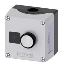
Enclosure for command devices, 22 mm, round, Enclosure material plastic, enclosure top part gray, 1 control point plastic, Recess for label, A=Pushbutton white, label: I, 1 NO, screw terminal, floor mounting, Label enclosed
