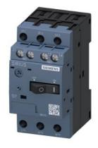
Circuit breaker size S00 for motor protection, CLASS 10 A-release 0.7...1 A N-release 13 A Screw terminal Standard switching capacity with transverse auxiliary switch 1 NO+1 NC
