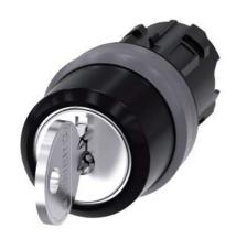
RONIS key-operated switch, 22 mm, round, plastic with metal front ring, lock number SB30, with 2 keys, 3 switch positions I-O-II, latching, actuating angle 2x45°, 10:30h/12h/13:30h, Key removal I+II, possible special locks: SB31, 421, 455, with laser labeling, lower case
