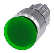
Illuminated mushroom pushbutton, 22 mm, round, metal, shiny, green, 30 mm, latching, pull-to-unlatch mechanism, Z=50-unit packaging
