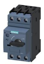
Special type Circuit breaker size S0 for motor protection, CLASS 10 A-release 18...25 A N-release 325 A Screw terminal Standard switching capacity Ambient temperature -50  $^\circ$ C 500 switching cycles
