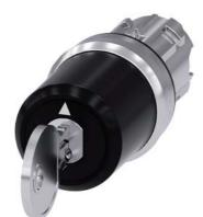
Key-operated switch BKS, 22 mm, round, metal, shiny, lock number S1, with 2 keys, 3 switch positions I-O-II, latching, actuating angle 2x45°, 10:30h/12h/13:30h, Key removal I+O+II, with laser labeling, inscription or symbol Customer-specific selection with SIRIUS ACT configurator (CIN)
