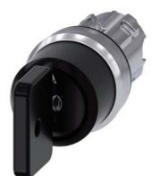
Key-operated switch O.M.R, 22 mm, round, metal, shiny, lock number 73034, black, with 2 keys, 3 switch positions I>O<II, momentary contact on the left, latching on the right, actuating angle 2x45°, 10:30h/12h/13:30h, Key removal II, Z=50-unit packaging
