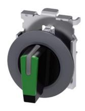
Selector switch, illuminable, 30 mm, round, Metal, matte, green, selector switch, short, front ring for flush installation, 3 switch positions I-O-II, latching, actuating angle 2x45°, 10:30h/12h/13:30h, with laser labeling, lower case
