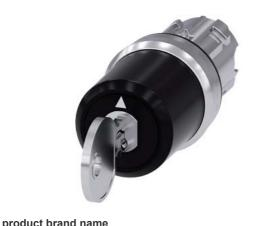
key-operated switch Siemens, 22 mm, round, metal, shiny, lock number SSG10, with 2 keys, 3 switch positions I-O-II, latching, actuating angle  $2x45^{\circ}$ , 10:30h/12h/13:30h, key removal I+II, with laser labeling, upper case and lower case, always upper case at beginning of line
