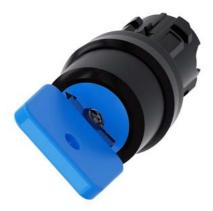
Key-operated switch O.M.R, 22 mm, round, plastic, lock number 73038, blue, with 2 keys, 2 switch positions O-I, latching, actuating angle  $90^\circ, 10:30h/13:30h$ , key removal O+I, with laser labeling, upper case and lower case, always upper case at the beginning of the word
