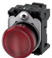
Indicator lights, 22 mm, round, plastic, red, lens, smooth, with holder, LED module with integrated LED 110 V AC, spring-type terminal, with laser labeling, upper case
