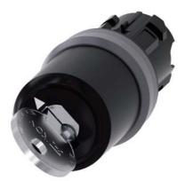
Key-operated switch IKON, 22 mm, round, plastic with metal front ring, lock number 360012K1, with 2 keys, 2 switch positions O<I, momentary contact type, Actuating angle 45°, 10:30h/12h, key removal O, with laser labeling, inscription or symbol Customer-specific selection with SIRIUS ACT configurator (CIN)
