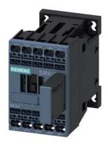
power contactor, AC-3 12 A, 5.5 kW / 400 V 1 NO, 24 V DC 0.7-1.25\* US, with varistor plugged on, 3-pole size S00, spring-type terminal not expandable with auxiliary switch
