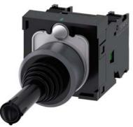
Coordinate switch, 22 mm, round, plastic with metal front ring, black, 2 switch positions, horizontal, momentary contact type, without mechanical interlocking in O position, with holder, 1 NO, 1 NO, screw terminal, with laser labeling, upper case and lower case, always upper case at the beginning of the word
