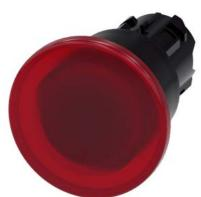
Illuminated mushroom pushbutton, 22 mm, round, plastic, red, 40mm, latching, pull-to-unlatch mechanism, with laser labeling, symbol number according to, ISO 7000 or IEC 60417
