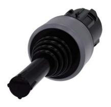
Coordinate switch, 22 mm, round, plastic with metal front ring, black, 4 switch positions, latching, without mechanical interlocking, with laser labeling, upper case and lower case, always upper case at beginning of line
