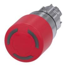
EMERGENCY STOP mushroom pushbutton, illuminable, 22 mm, round, metal, shiny, red, 30 mm, positive latching, acc. to EN ISO 13850, rotate-to-unlatch, with laser labeling, upper case and lower case, always upper case at beginning of line
