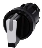
Selector switch, illuminable, 22 mm, round, plastic, white, selector switch, short, 3 switch positions I>O<II, momentary contact type, actuating angle 2x45°, 10:30h/12h/13:30h, with laser labeling, lower case
