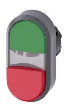
Illuminated twin pushbutton, 22 mm, round, plastic with metal front ring, red, green, pushbuttons, flat and raised, with laser labeling, symbol number according to, ISO 7000 or IEC 60417
