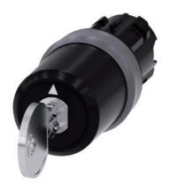
Key-operated switch BKS, 22 mm, round, plastic with metal front ring, lock number S1, with 2 keys, 3 switch positions I-O-II, latching, actuating angle 2x45°, 10:30h/12h/13:30h, Key removal I+O+II, with laser labeling, upper case
