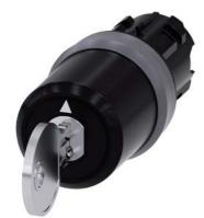
Key-operated switch BKS, 22 mm, round, plastic with metal front ring, lock number S1, with 2 keys, 3 switch positions I-O<II, left latching, right momentary contact type, actuating angle 2x45°, 10:30h/12h/13:30h, key removal O+I, with laser labeling, Customer-specific selection with SIRIUS ACT configurator (CIN)
