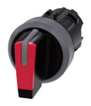
Selector switch, illuminable, 22 mm, round, plastic with metal front ring, red, selector switch, short, 3 switch positions I>O<II, momentary contact on the left, latching on the right, actuating angle 2x45°, 10:30h/12h/13:30h, with laser labeling, upper case
