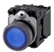
Illuminated pushbutton, 22 mm, round, plastic with metal front ring, blue, pushbutton, flat, momentary contact type, with holder, 1NO, LED module with integrated LED 230 V AC, screw terminal, with laser labeling, lower case
