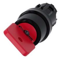
Key-operated switch O.M.R, 22 mm, round, plastic, lock number 73037, red, with 2 keys, 2 switch positions O-I, latching, actuating angle 90°, 10:30h/13:30h, Key removal O Z=50-unit packaging
