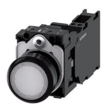
Illuminated pushbutton, 22 mm, round, plastic, white, pushbutton, flat, momentary contact type, with holder, 1 NO+1 NC, LED module with integrated LED 110 V AC, spring-type terminal, Z=20-unit packaging
