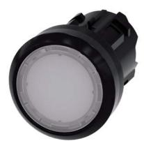
Illuminated pushbutton, 22 mm, round, plastic, white, pushbutton, flat, latching, Push-to-release mechanism, with laser labeling, upper case and lower case, Always upper case at the beginning of the word
