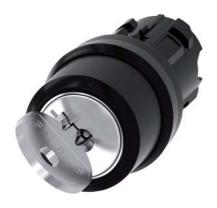
RONIS key-operated switch, 22 mm, round, plastic, lock number SB30, with 2 keys, 2 switch positions O-I, latching, actuating angle  $90^\circ, 10:30h/13:30h,$  key removal O+I, possible special locks: SB31, 421, 455, with laser labeling, upper case and lower case, always upper case at the beginning of the word
