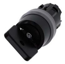
Key-operated switch O.M.R, 22 mm, round, plastic with metal front ring, lock number 73034, black, with 2 keys, 2 switch positions O-I, latching, actuating angle 90°, 10:30h/13:30h, key removal I, with laser labeling, lower case
