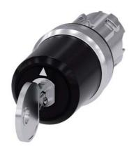
key-operated switch Siemens, 22 mm, round, metal, shiny, lock number SSG10, with 2 keys, 3 switch positions I-O-II, latching, actuating angle 2x45°, 10:30h/12h/13:30h, key removal I+II, Z=50-unit packaging
