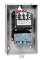
Non-reversing motor starter, Size 1, Three phase full voltage, Solid-state overload relay, OLR amp range 0.25-1A, Non-combination type, Enclosure type 1, Indoor general purpose use, Standard width enclosure
