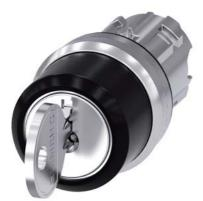
RONIS key-operated switch, 22 mm, round, metal, shiny, lock number SB30, with 2 keys, 3 switch positions I>O<II, momentary contact on the left, latching on the right, actuating angle 2x45°, 10:30h/12h/13:30h, key removal O, possible special locks: SB31, 421, 455, with laser labeling, inscription or symbol Customer-specific selection with SIRIUS ACT configurator (CIN)
