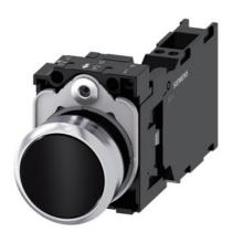
Pushbutton, 22 mm, round, metal, shiny, black, pushbutton, flat, momentary contact type, 1 NO+1 NC, spring-type terminal, Z=20-unit packaging
