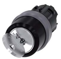
RONIS key-operated switch, 22 mm, round, plastic with metal front ring, lock number SB30, with 2 keys, 2 switch positions O<I, momentary contact type, Actuating angle 45°, 10:30h/12h, key removal O, possible special locks: SB31, 421, 455, with laser labeling, lower case
