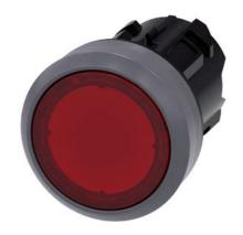
Illuminated pushbutton, 22 mm, round, plastic with metal front ring, red, pushbutton, flat, latching, Push-to-release mechanism, with laser labeling, upper case
