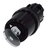
Key-operated switch BKS, 22 mm, round, plastic, lock number S1, with 2 keys, 2 switch positions O-I, latching, actuating angle  $90^\circ$ , 10:30h/13:30h, key removal O+I, with laser labeling, lower case
