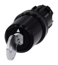
key-operated switch Siemens, 22 mm, round, plastic, lock number SSG10, with 2 keys, 3 switch positions I>O<II, momentary contact on the left, latching on the right, actuating angle 2x45°, 10:30h/12h/13:30h, key removal O, with laser labeling, upper case and lower case, always upper case at beginning of line
