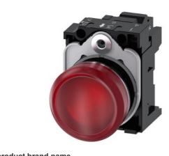
Indicator lights, 22 mm, round, metal, shiny, red, lens, smooth, with holder, LED module with integrated LED 110 V AC, spring-type terminal, with laser labeling, inscription or symbol Customer-specific selection with SIRIUS ACT configurator (CIN)
