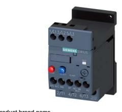
Overload relay 0.70...1.0 A Thermal For motor protection Size S00, Class 10 Stand-alone installation Main circuit: Screw Auxiliary circuit: Screw Manual-Automatic-Reset
