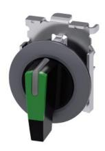
Selector switch, illuminable, 30 mm, round, Metal, matte, green, selector switch, long, front ring for flush installation, 3 switch positions I-O-II, latching, actuating angle 2x45°, 10:30h/12h/13:30h, with laser labeling, upper case
