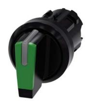
Selector switch, illuminable, 22 mm, round, plastic, green, selector switch, short, 3 switch positions I>O<II, momentary contact on the left, latching on the right, actuating angle 2x45°, 10:30h/12h/13:30h, with laser labeling, upper case and lower case, always upper case at beginning of line
